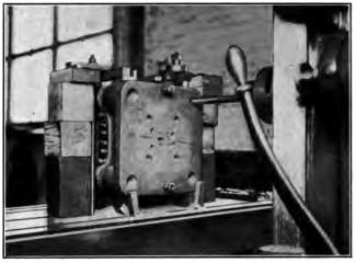
Fig. 15. Boring Sub-press Die Guide-pin Holes
